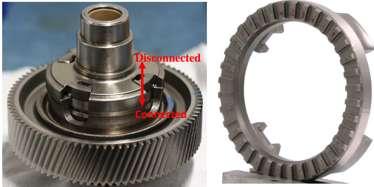
Figure 22: Disconnecting differential (left) and disconnecting disc (right)
