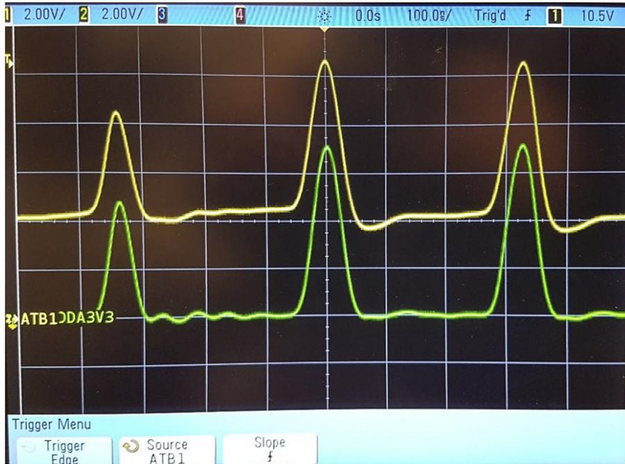
Figure 2.9: Pulse generated by function generator (green: pulse, yellow: 5V DC and pulse).
