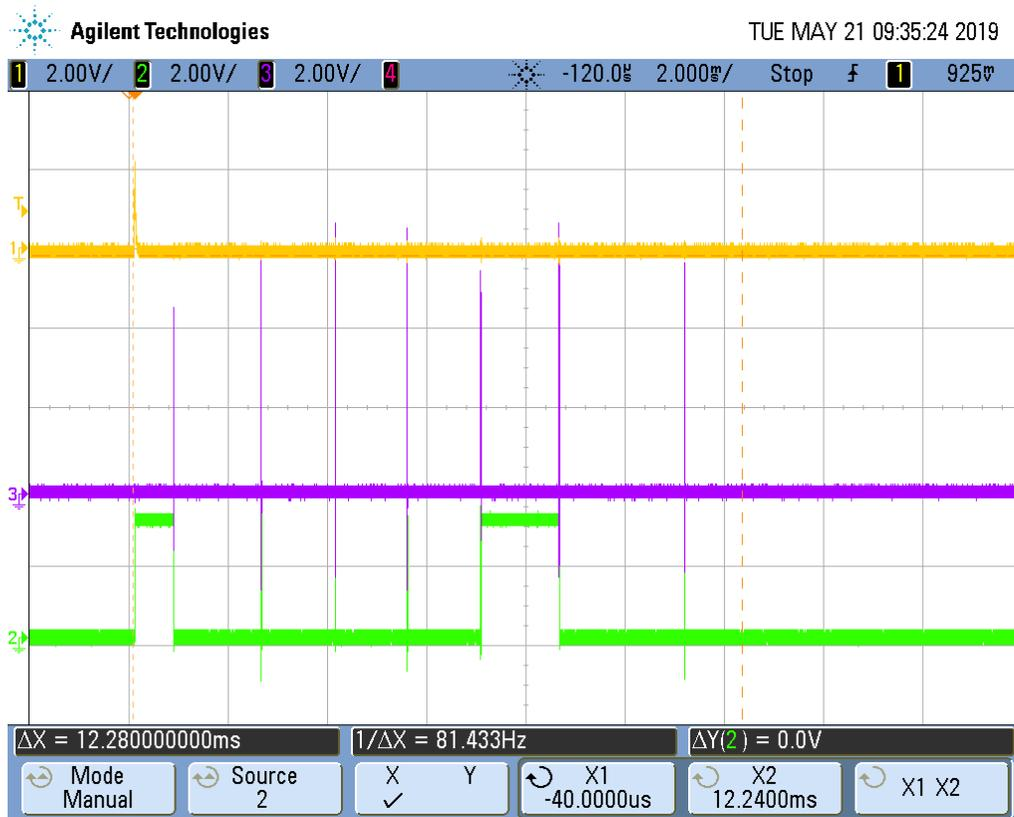
Figure 4.18: Example of SPI communication.
