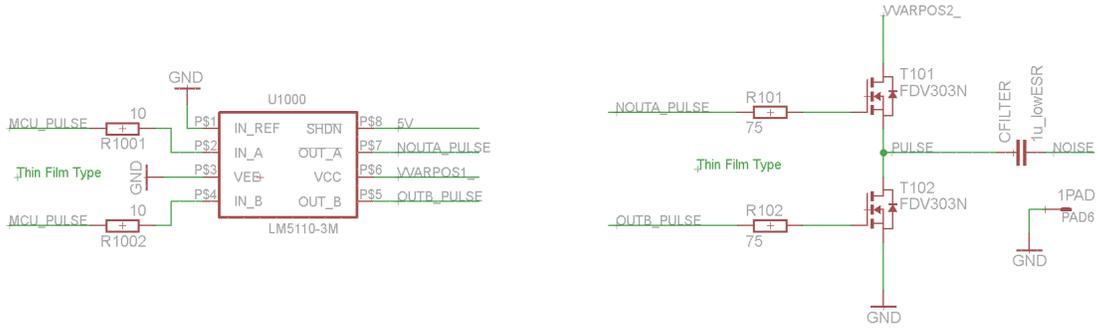
Figure 4.14: Gate driver IC and half-bridge circuit.
