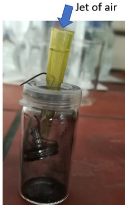
Figure 6.4: Sampling by air-jetting
