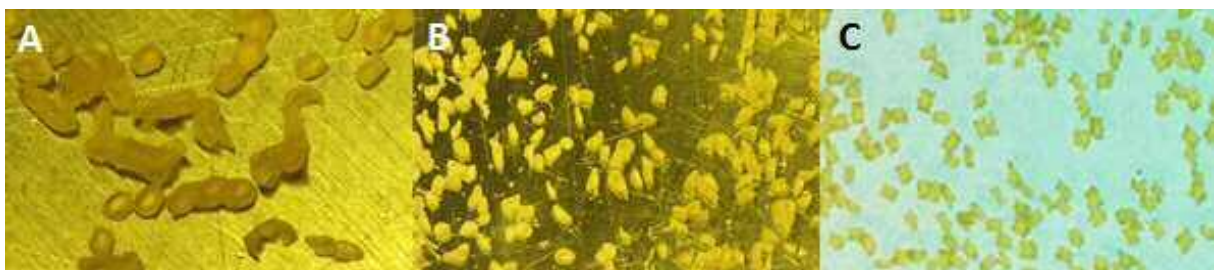
Figure 3-8. Two types of pelletization problems in die-face pelletization: Pellet chains (A) and tailed and irregularly shaped pellets (B). Cylindrical pellets from strand pelletization (C).
