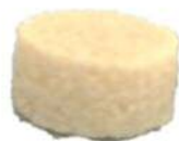
Figure 5-2. Tablet compressed at 5 kN from NMD-pellets after 40 min of disintegration testing.
