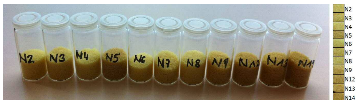
Figure 3-10. Pellets from all screening DoE runs, with different levels of HPMC browning for pellets produced at different screw speeds. Right: picture regions used for colorimetric analysis.
