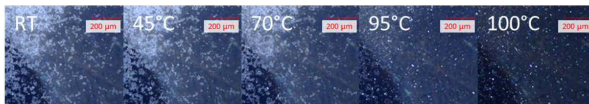
Figure A-1. Polarized light hot-stage microscopy images of EE particles recorded during a heating ramp at 5 K/min and 40°C to 120°C. Softening of the particles is evidenced by an increasing transparency of particles after T g at 48°C. Coalescence and flow of the particles is observed only at above 95°C, indicating a relaxation of main block chains in the polymers.
