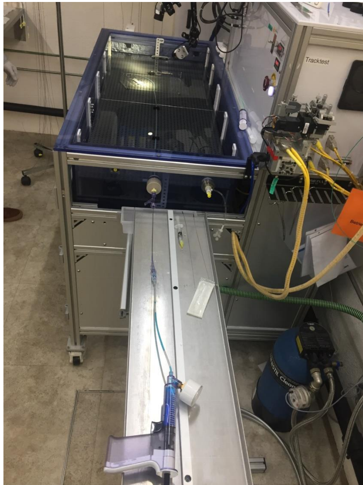
Figure 28: Test setup for performing stent implantations
