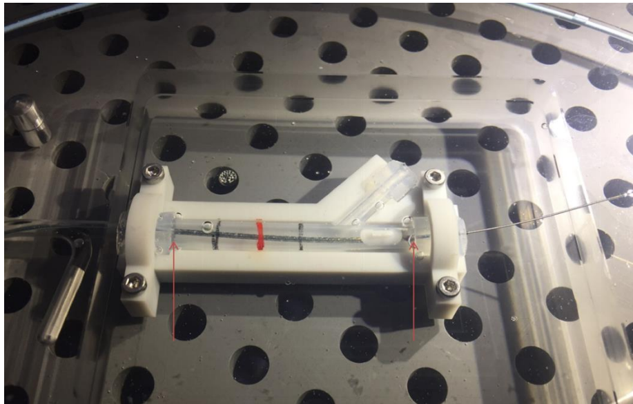
Figure 26: Optimal placement of the delivery system at the distal and proximal vessel ends
