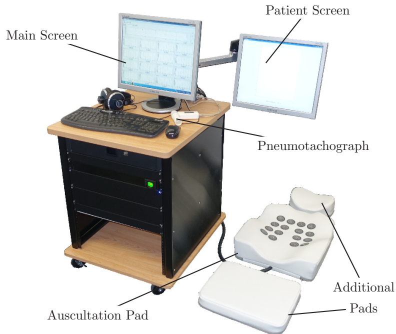
Figure 3.3: Mobile lung sound recording device containing the auscultation pad and the additional components.
