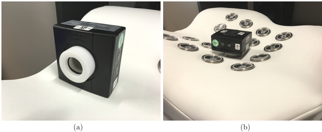
Figure 3.5: Calibration with a Brüel & Kjær sound calibrator Type 4231: a) shows the calibrator including the adapter and b) its attachment to a LST.
