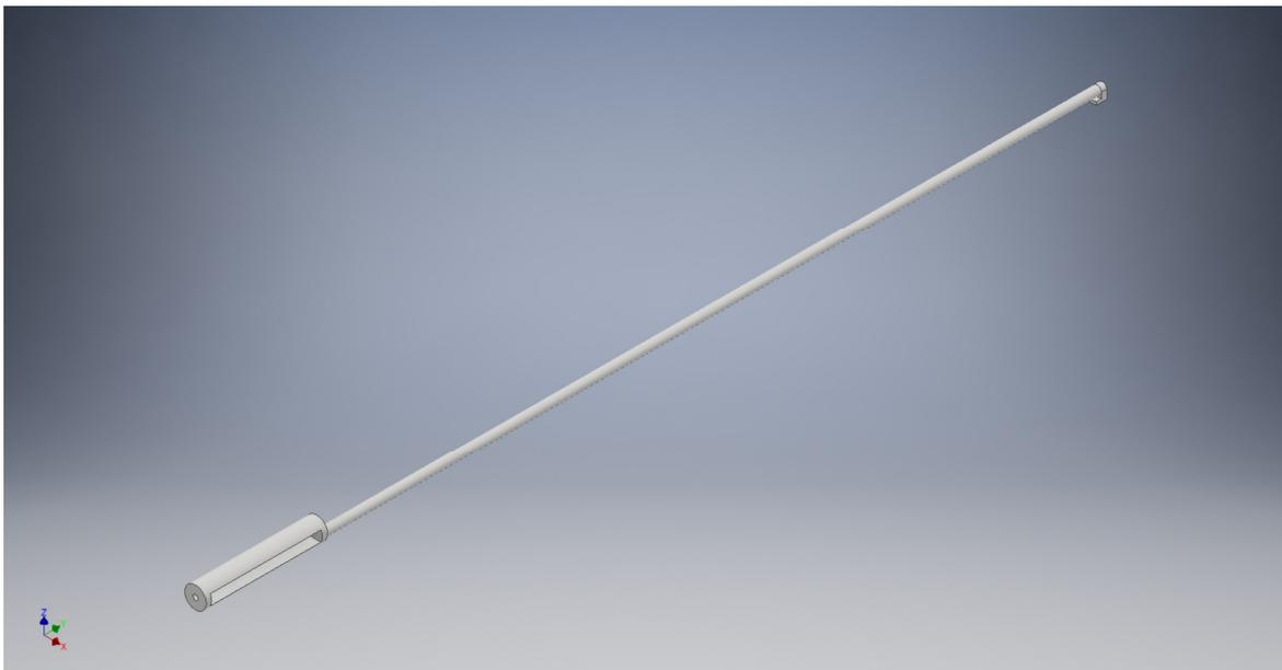
**Figure 3-2 Isometric view of the second prototype. The dimensions are identical to the first prototype except for the inner chamber. The chamber is a 2 mm wide and 21 mm high rectangular hole. The exact dimensions can be found in the appendix. The prototype was designed using Autodesk Inventor Professional 2019. (Figure 6-2 and Figure 6-3)**
