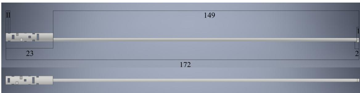
**Figure 6-2** The exact dimensions of the first prototype from the x- and z-view. These dimensions were also taken for the second prototype, except for the size of the chamber.
