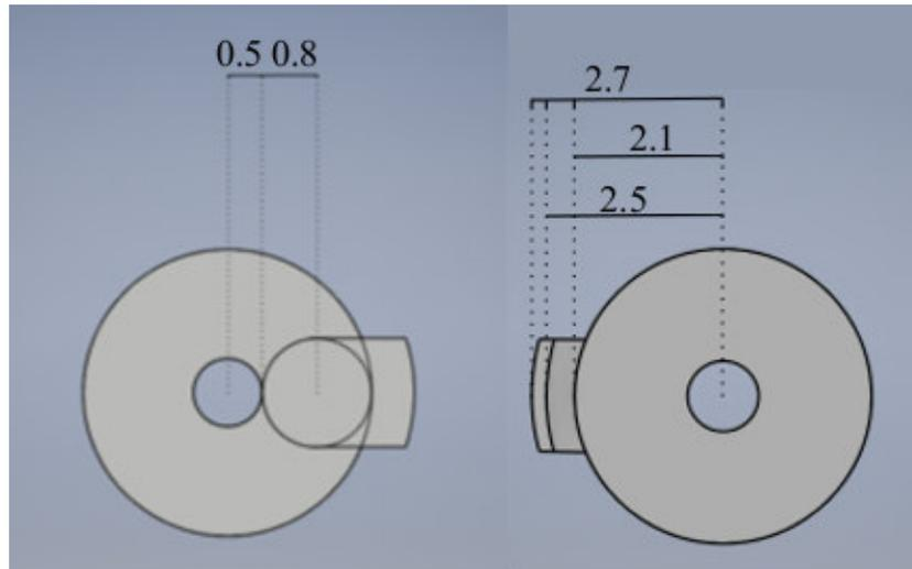
**Figure 6-3** The exact dimensions of the first prototype from the y-views. These dimensions were also taken for the second prototype.
