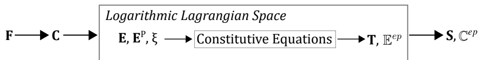
Figure 4.3. Approach for the solution algorithm for rate-independent plasticity in logarithmic Lagrangian strain space (Cf. Ulz [33])
