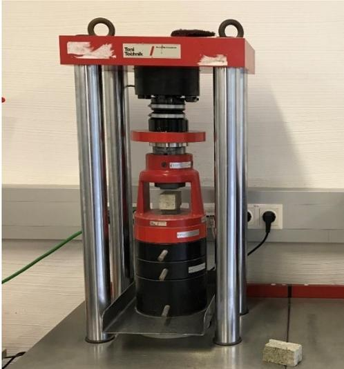
Figure 15: Compressive Strength-testing machine "ToniNORM" (300kN)
