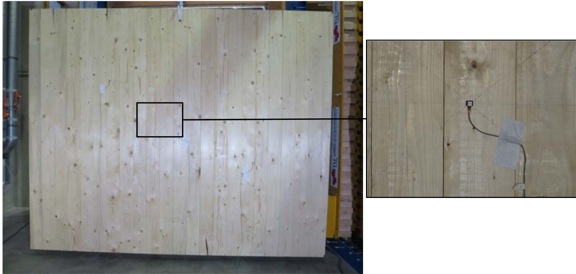
Figure 5.4: Single CLT - specimen and test setup – 3s CLT wall
