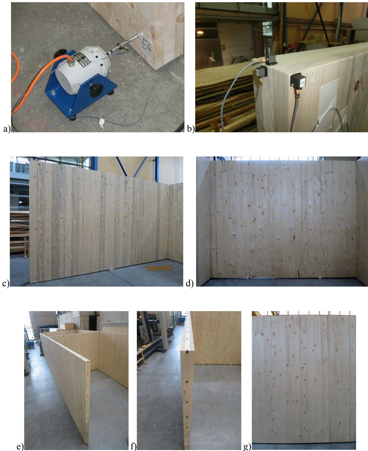
Figure 4.49: Measurements of vibration components on a construction of a H-Shape – a) Shaker excitation and measurement of the induced force; b) reference sensors for out-of-plane and in-plane components; c) measurement positions of out-of-plane components of wall 4; d) measurement positions for wall 3 (separation wall); e) f) measurement positions for in-plane components; g) measurement positions for in-plane components of the separation wall (attachment on screws);
