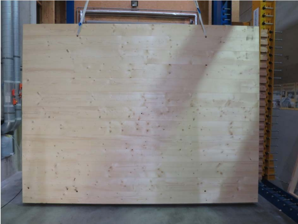
Figure 5.6: Single CLT 5s floor – specimen and test setup
