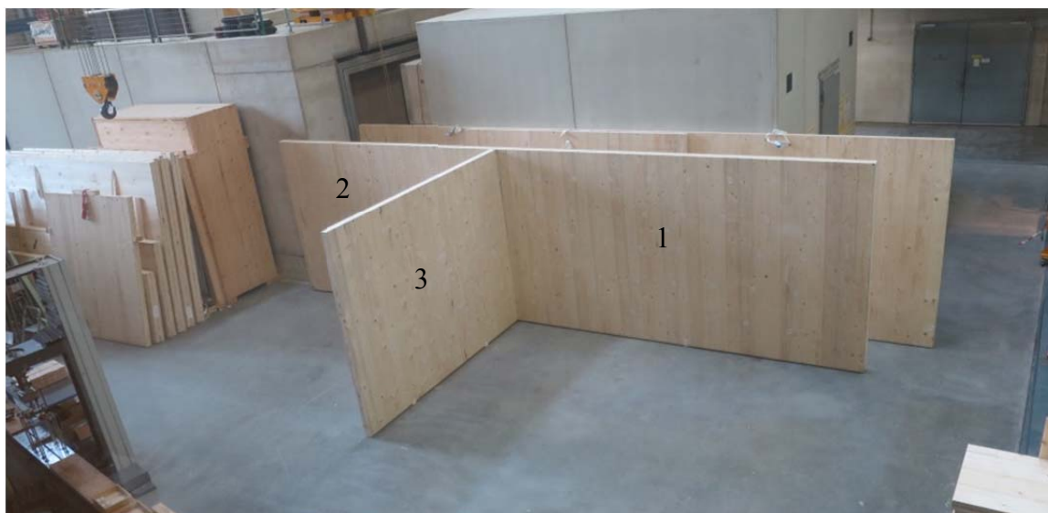
Figure 3.11: Test setup for measurements on a T-shaped mock-up without wall 4
