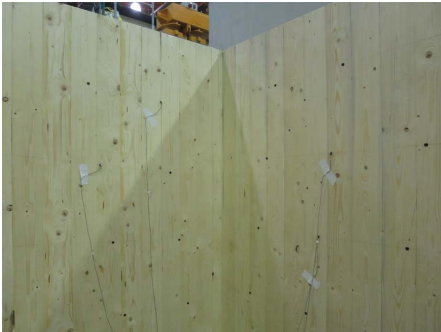
Figure 5.11: mounting of the acceleration sensors during measurements
