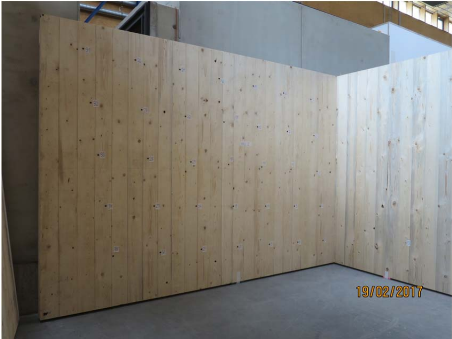
Figure 5.13: Measurement positions of out-of-plane components of wall 2
