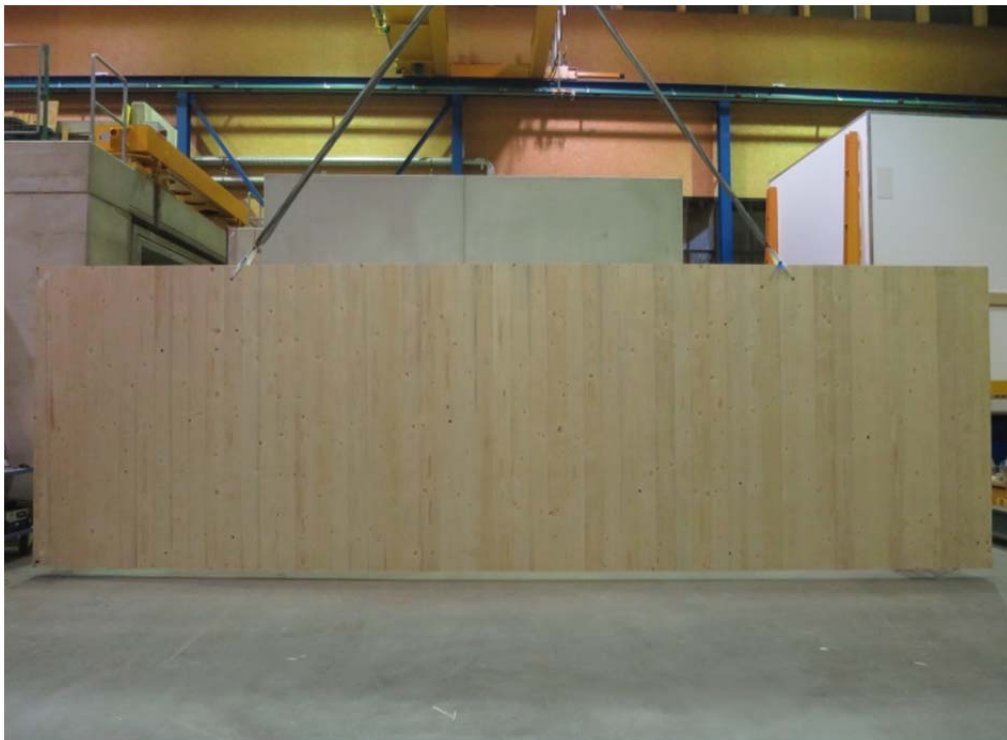
Figure 5.5: Single CLT - specimen and test setup – 5s CLT wall
