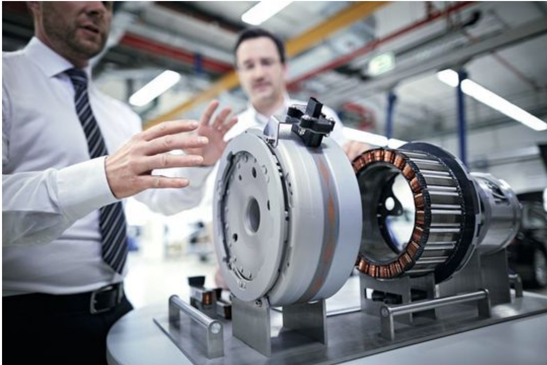
Figure 36. The electric engine of E-Tron Quattro - the 1 st purely electric model by Audi [50]
