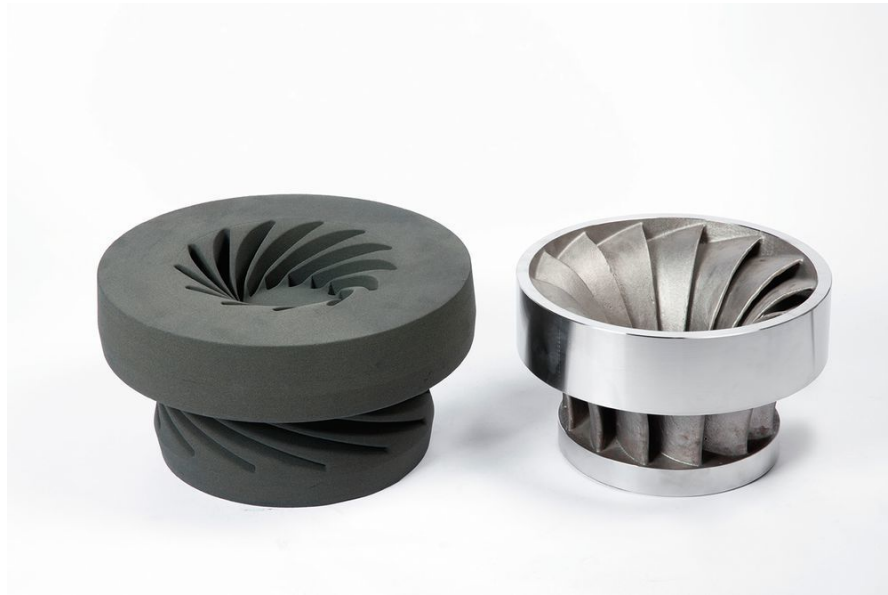
Figure 51. Tool-free production of an impeller: 3D-printed sand core (left) and the final casting (right) [57]
