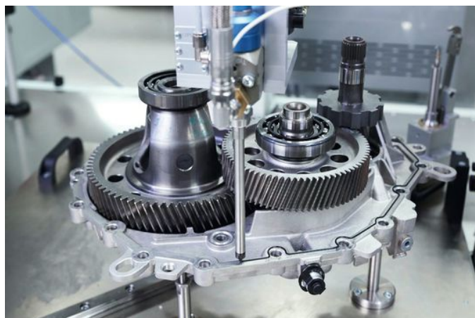
Figure 35. Casting and steel: prototyping of the prospective gear of an electric drivetrain [46]
