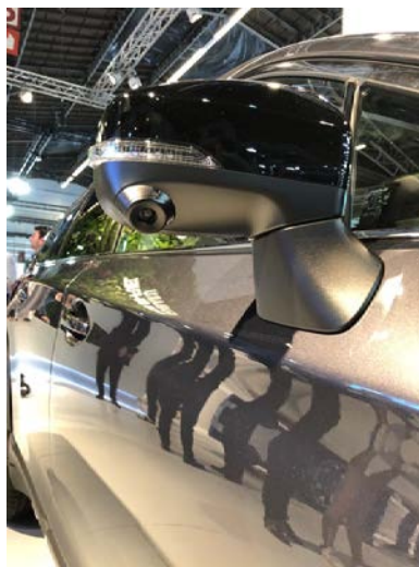
Figure 31. Subaru, external camera for 360° view as seen in Automobile Barcelona Motor Show, 2019
