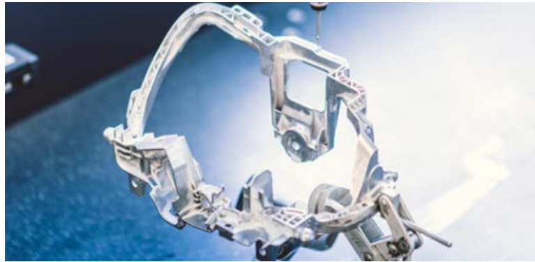
Figure 6. Support frame for lighting and electric system [1]
