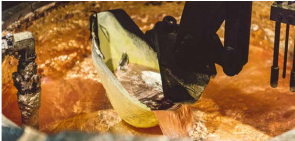
Figure 13. Centralized melting machinery. Temperature maintenance - a key process in die casting [1]
