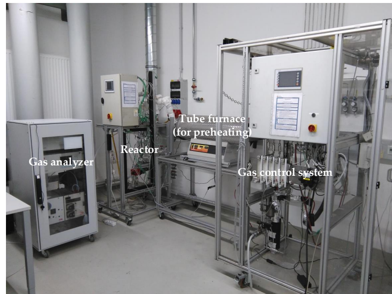
Figure 3.24: SR test rig including reactor, gas control system, tube furnace for preheating and gas analyzer.
