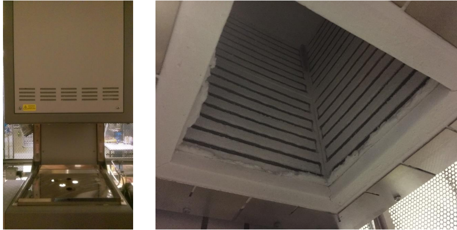
Figure 3.34: Left: top-hat furnace front view; Right: interior view with heating coils.
