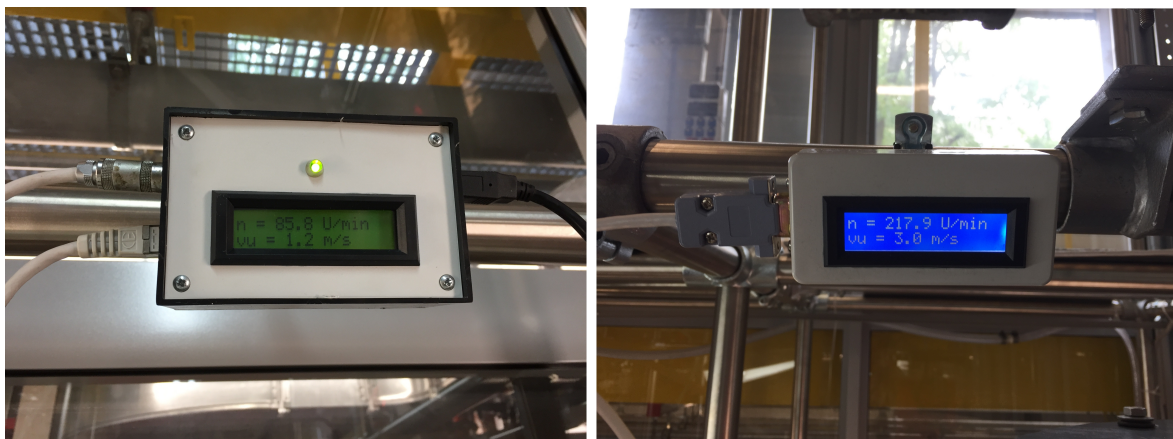
Fig. 3-11: left: Display next to the control box showing rpm and circumferential speed; right: Display next to the gear motor for coarse adjustment of rotational speed
