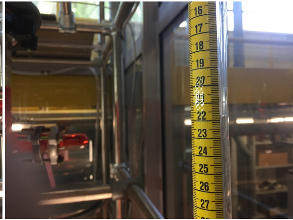
Fig. 5-3: Height of the continuous phase h_1 in the level gauge
