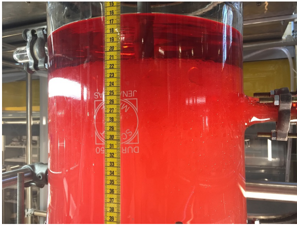
Fig. 5-2: Height of phase interface h_2
