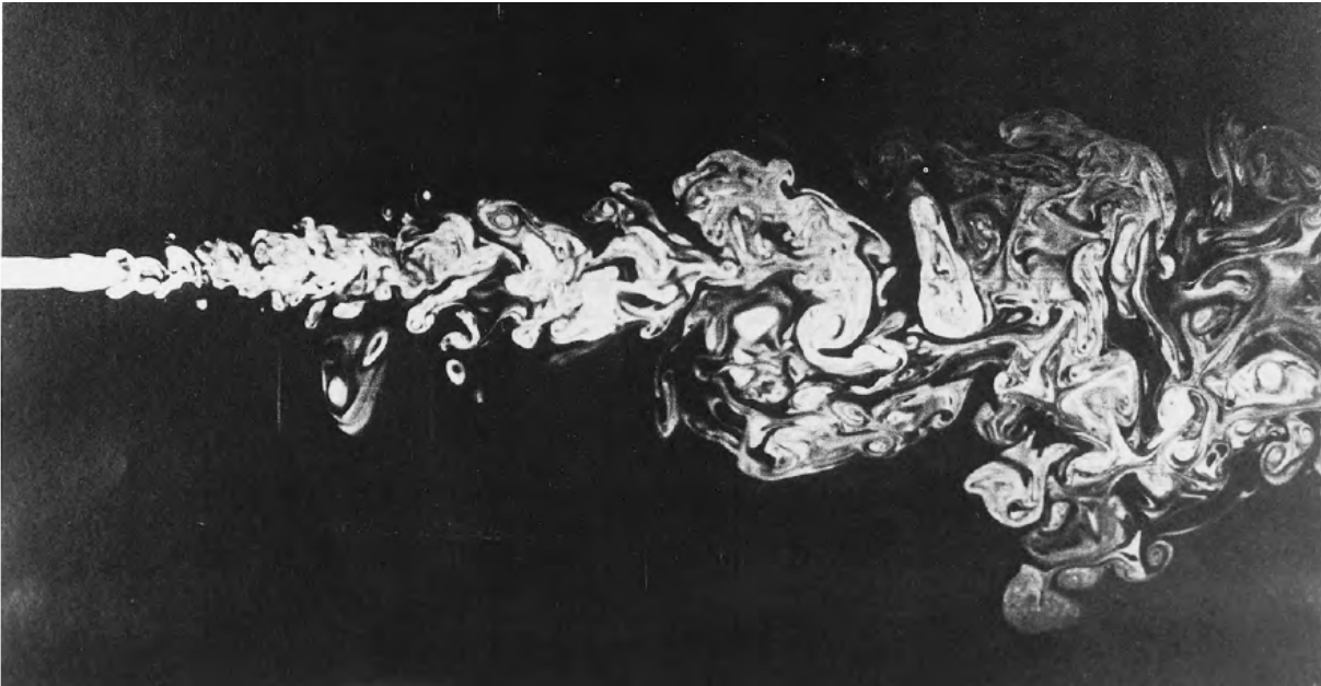
Fig. 2.2: Visualization of turbulence of a jet flow [41]
