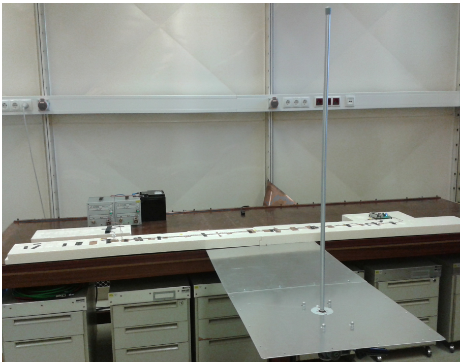
Figure 2.5.: Test setup in a non-certified shielded enclosure without absorbers used for the red curve of Fig. 2.3. The photo was taken in the EMC lab of the Institute for Electronics at Graz University of Technology where most of the experiments for this thesis were conducted.
