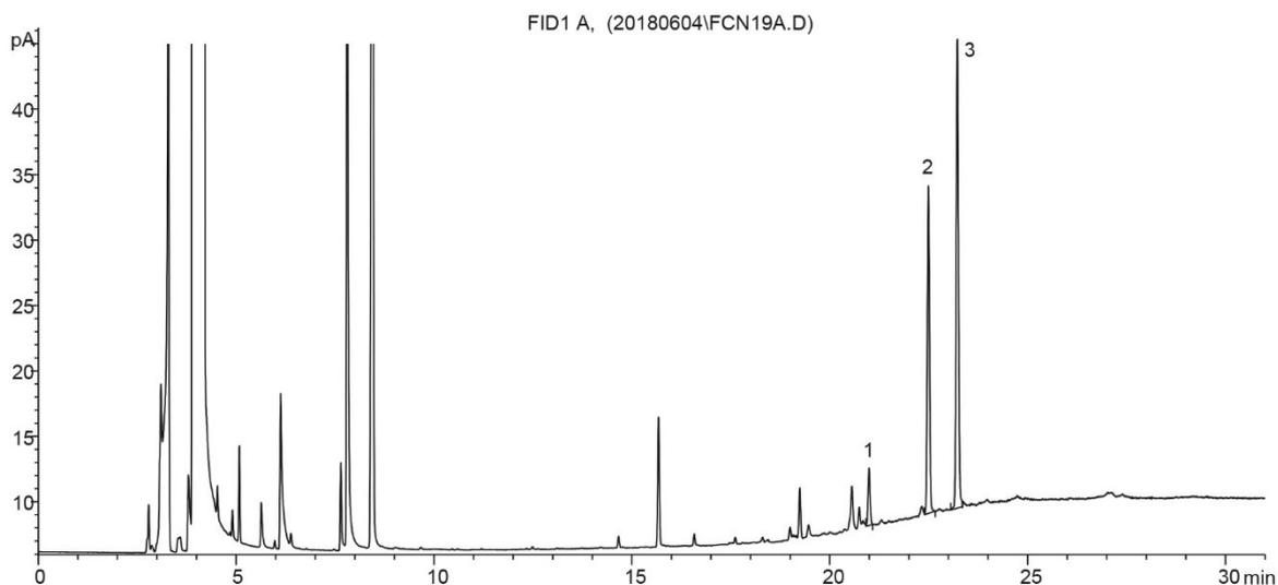
Figure 37. GC-FID of the second eluting fraction of the sample "Fraction I"; 1 – C16 amide; 2 – C18:1 amide; 3 – C19 amide
