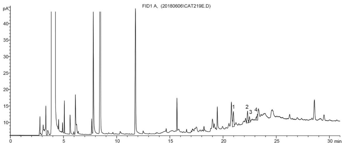
Figure 39. GC-FID of the second eluting fraction of the sample "Fraction I"; 1 – C16 amide; 2 – C18:1 amide; 3 – C18 amide; 4 - C19 amide
