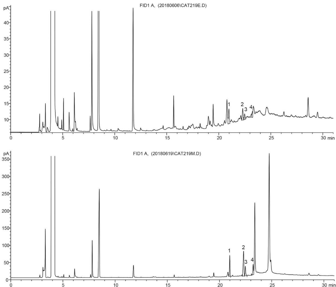
Figure 42. Comparison of chromatograms obtained with 1 g of sample (up) and 0.5 g of sample (down)
