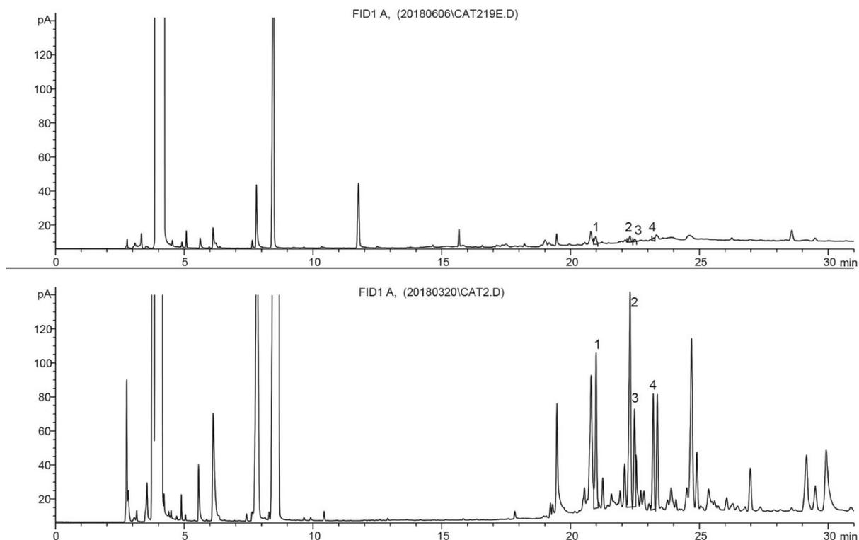
Figure 40. Comparison of chromatograms obtained with the new (up) and old (down) method
