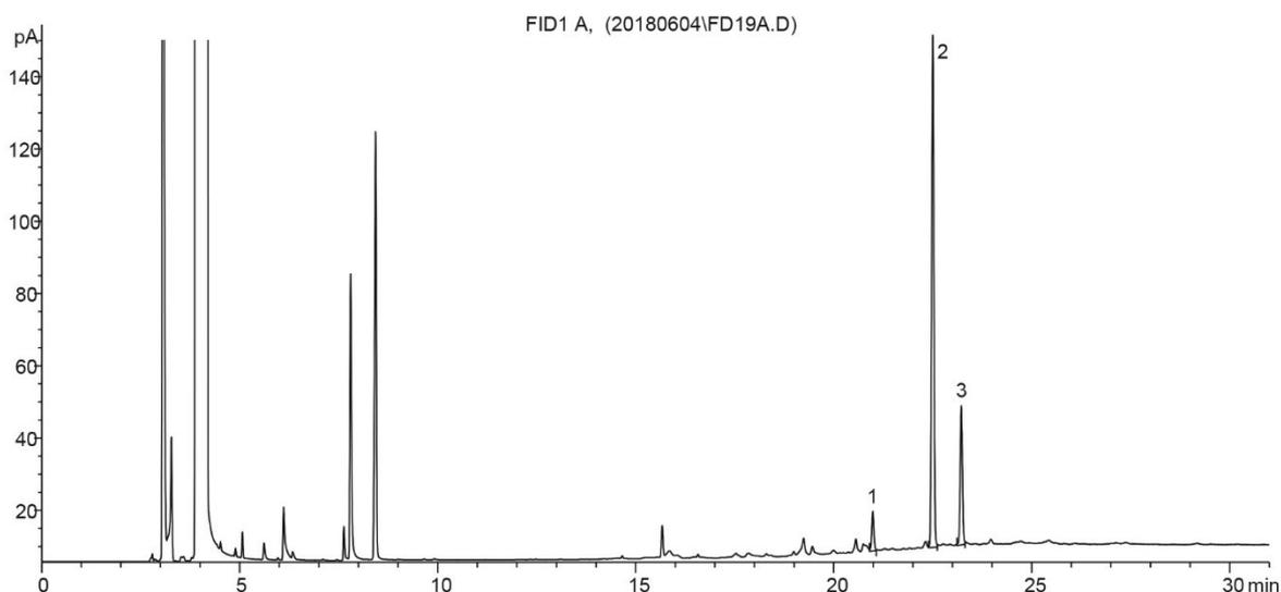
Figure 35. GC-FID of the second eluting fraction of the sample "Feed 18-18"; 1 – C16 amide; 2 – C18:1 amide; 3 – C19 amide
