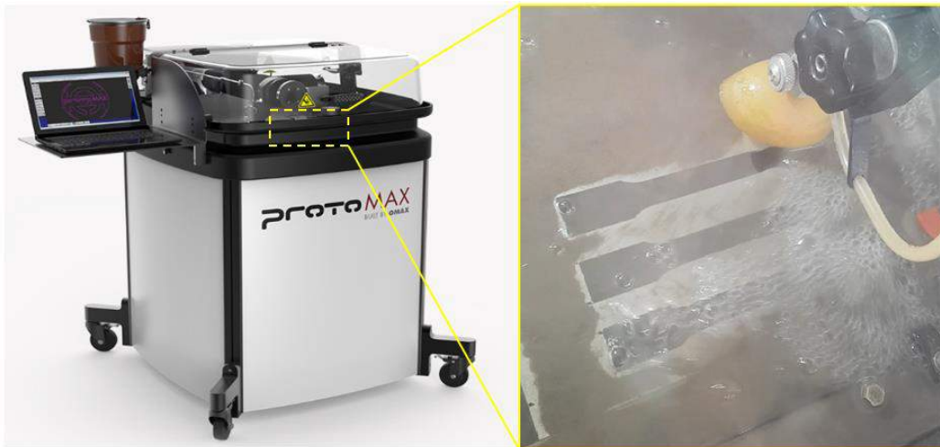
Figure 25: Sample preparation with the waterjet cutter built by OMAX [84]
