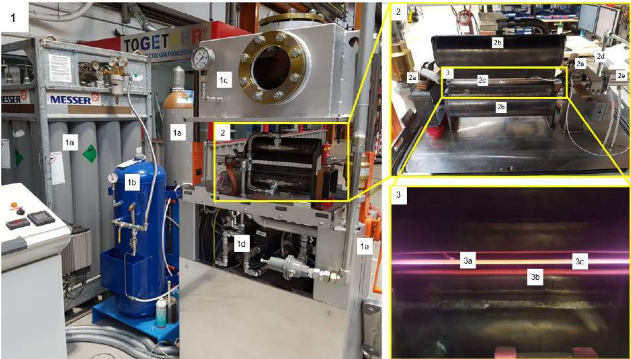
Figure 41: EBNER's SimCAL 3.0 continuous heat treatment simulation tool (1a: gas bottles, 1b: puffer tank, 1c: cover, 1d: control unit, 1e: crank handle, 2a: Cu brackets, 2b: frame, 2c: cold steel stripe, 2d: N purging tube, 2e: clamping cylinder, 3a: thermocouple, 3b: slits, 3c: heated steel stripe)
