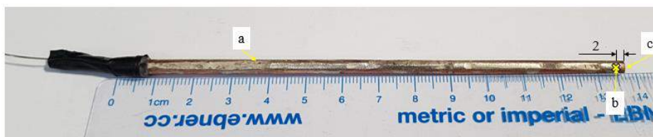
Figure 51: Sheath thermocouple placed on the inside of a Cu nail
