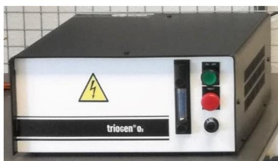
Figure 13: SUEZ - Triogen<sup>®</sup>O<sub>3</sub> LAB2B ozone generator with corona discharge
