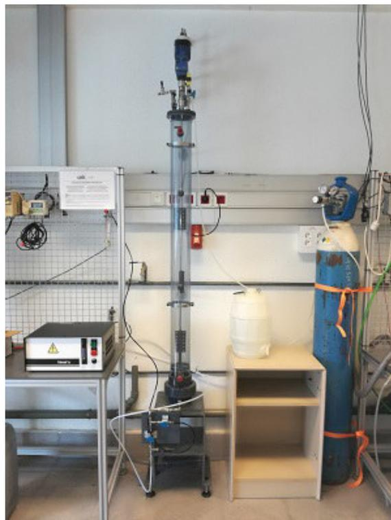
Figure 17: Ozonation reactor set up in the CEIT laboratory
