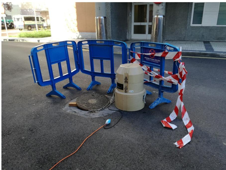
Figure 12: Set up of the sampling device Tomamuestra SIGMA 900 at the hospital (Donostiako Uniberstitate Ospitalea)
