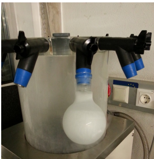
Figure 3.20: Process of lyophilization.
