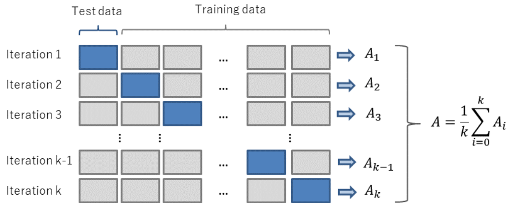
Figure 7.2.: The cross validation method is shown in the graphic. Initially the data set is randomly split into k-folds, where k has to be chosen accordingly. One fold is chosen to be the test set, whereas the residual k-1 folds represent the training set. The model is trained with k-1 folds, tested with the last fold and discarded. These steps are done for each iteration. The final evaluation is the average over all trained models in each of the k iterations.
