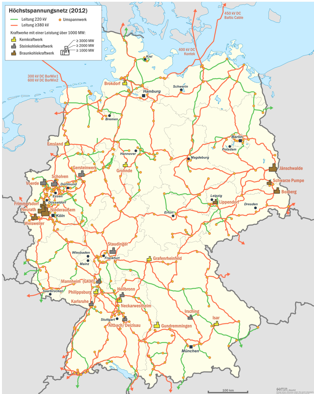
Figure 2.1: High-voltage grid map of Germany with high-voltage power lines above 220 kV and power plants above 1000 MW electric power. (2012)
