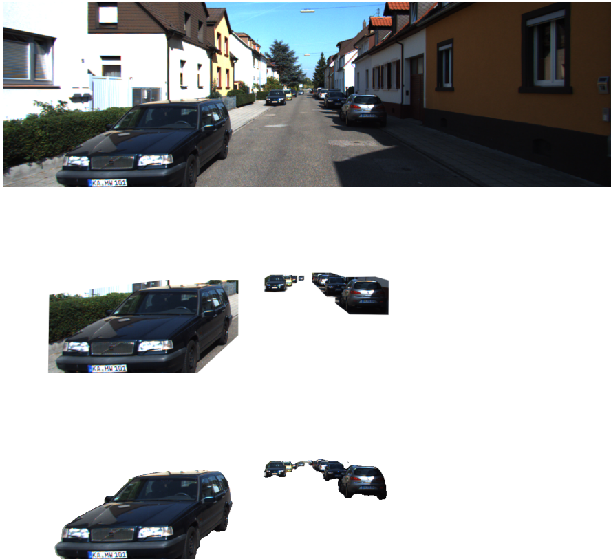
FIGURE 4.2: Top: Original image. Middle: Segmented target objects using groundtruth 3D bounding boxes. Bottom: Segmented target objects using VideoPropLabelRelax [56] masks
