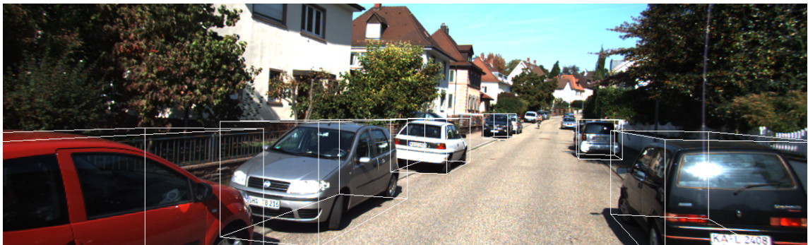
FIGURE 2.7: Example 3D bounding box groundtruth annotations from the KITTI dataset. Image taken from [22].
