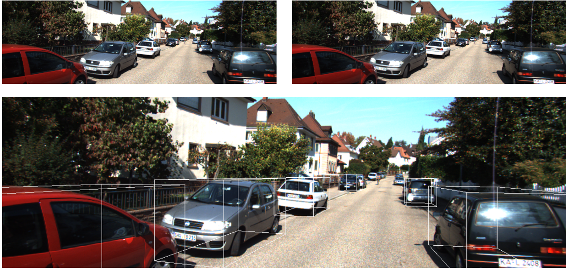
FIGURE 1.2: Example from the KITTI dataset. Top: Stereo input images. Bottom: 3D bounding boxes of objects projected into the input image.
