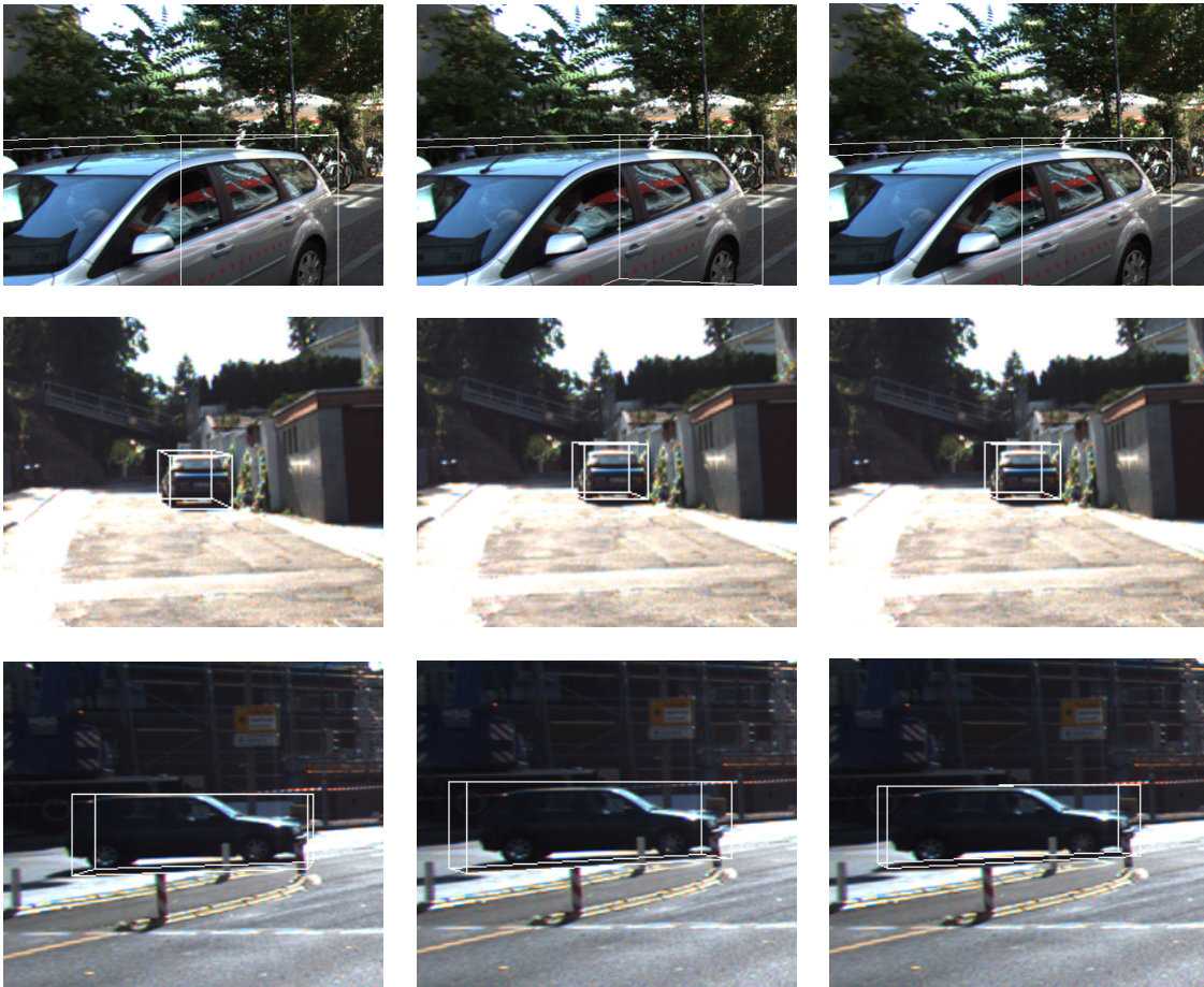
FIGURE 6.3: Comparison of qualitative results with different modifications applied. From left to right: groundtruth annotation, results from model with integrated object masks, results from end-to-end model with integrated object masks
