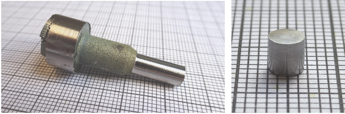
FIGURE 2.13.: Depiction of the sample preparation (first stage) on the lathe. The raw sample material (in this case a tensile test sample made from 3D-printed Ti6Al4V; see chapter 3, section 3.2.2) is first turned to a round rod (left) with a certain diameter. Using the room temperature density, the length needed for a cylinder of target size/mass is calculated and then parted off the rod (right). By preparing sample cylinders with (almost) equal diameter and length, instabilities in levitation during melting can be reduced (compared to other initial sample geometries like discs).
