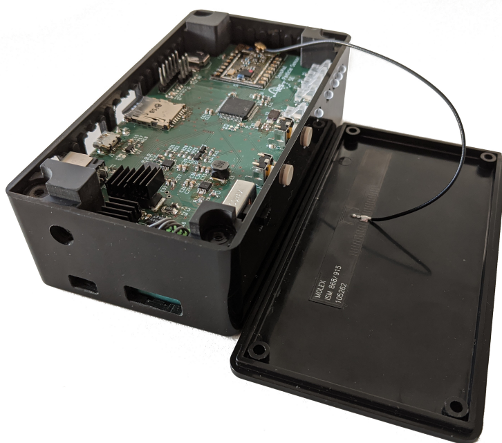
Figure 4.1: The fully assembled sensor node with the lid open.
