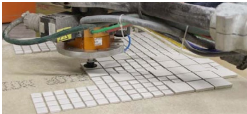
Abb.49: Robotic Tile Placement
