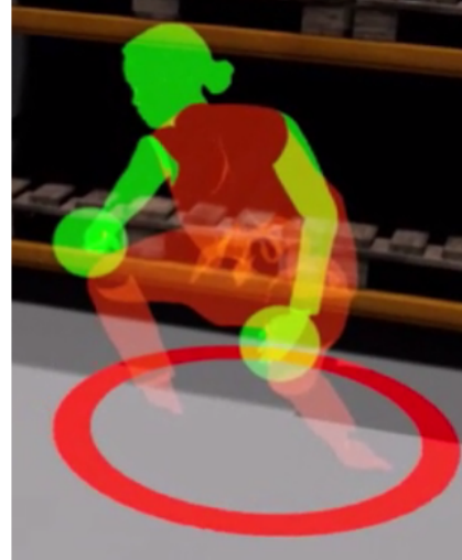
Figure 4.16: An avatar visualizes the pose filter. This avatar is a copy of the user's avatar and precisely reconstructs the user's pose in the evaluation. The partial OWAS results are visualized by coloring the corresponding body parts. The carried object is symbolized by two spheres that are located at the user's hands. The circle on the floor, that surrounds the avatar, represents the grade for the overall pose. The table on the right shows the color grading system.
