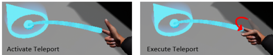
Figure 4.5: The picture on the left shows the user performing the gun gesture. This gesture activates the teleporter. The teleporter visualizes the destination point and its distance to the user. The user can control this destination point with the index finger. The right picture shows the user performing the gun trigger gesture. This gesture needs to be performed within a short time frame after the gun gesture to execute the teleport. After the gun trigger gesture is performed, the user teleports to the chosen destination point.
