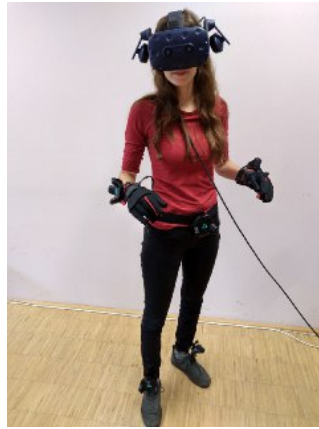
Figure 4.23: A user with the full setup: HTC Vive Pro, Manus Gloves and five Vive trackers, placed on the pelvis, each wrist and each ankle.
