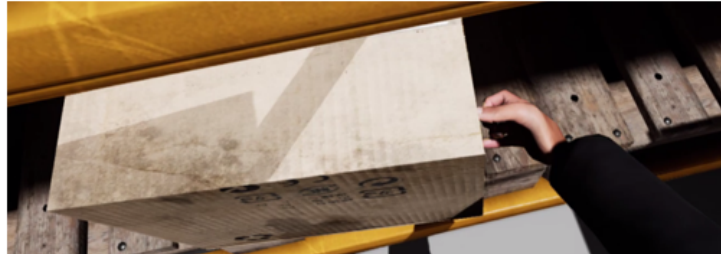
Figure 4.6: The user can pick up objects by performing a grab gesture. As long as the user uses this gesture, objects can be carried.
