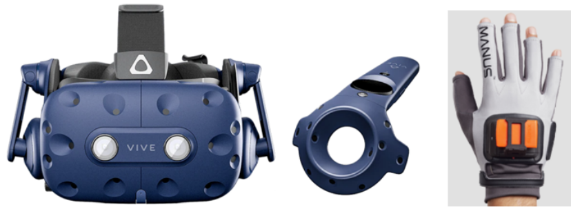
Figure 2.4: The pictures show a HMD (left) and a hand held-controller (middle) ( HTC Vive 2020). A glove from Manus Gloves (2021) is shown on the right.
