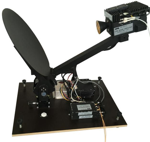
**Figure 1.1:** Pico terminal as used in the lab exercises. The antenna dish can be manually aligned in all directions.
