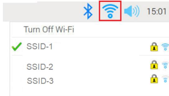
**Figure A.10:** Wi-Fi settings of the RaspberryPi. With a left mouse click on the Wi-Fi symbol in the taskbar, a list of available Service Set Identifiers (SSIDs) is shown. It is recommended to set up a hotspot with a smartphone and select the configured hotspot name from the list.
