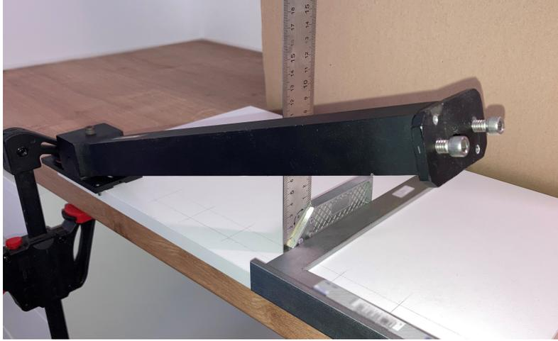
**Figure 4.1:** Setup to determine the antenna offset using Methods 2 & 3. With a clamp, the feed arm is hold in place. One angle is used as a stop and a second angle is used to measure the height between the bottom of the feed arm and the white plate. Markings on the left and the right side at a distance  $\Delta_x$  of 150 mm on the white plate indicate the measuring positions.
