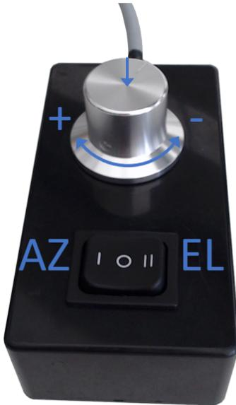
**Figure A.12:** Manual control panel for manual antenna adjustments. A switch for axis selection and a rotary encoder are the main components. Positive axis adjustments are made with the rotary encoder in clockwise direction. Pressing the button of the rotary encoder changes between three different step modes.
