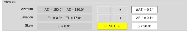
**Figure A.13:** *SET* button to change the skew angle. For correct azimuth and elevation calculations the manually set skew angle must be configured. In this case, a skew angle of 90° was configured, but not set. This is visualized with the yellow highlighted *SET* button. When clicking the *SET* button, the skew angle (named  $\beta$ ) is also set to 90° and the values for  $AZ$  and  $EL$  are changing, according to the configured skew angle.
