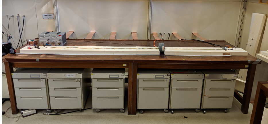
Figure 2.1.: Test setup for BCI substitution method after ISO 11452-4:2011. This photo was taken at the EMC Lab of the Institute of Electronics at TU Graz.
