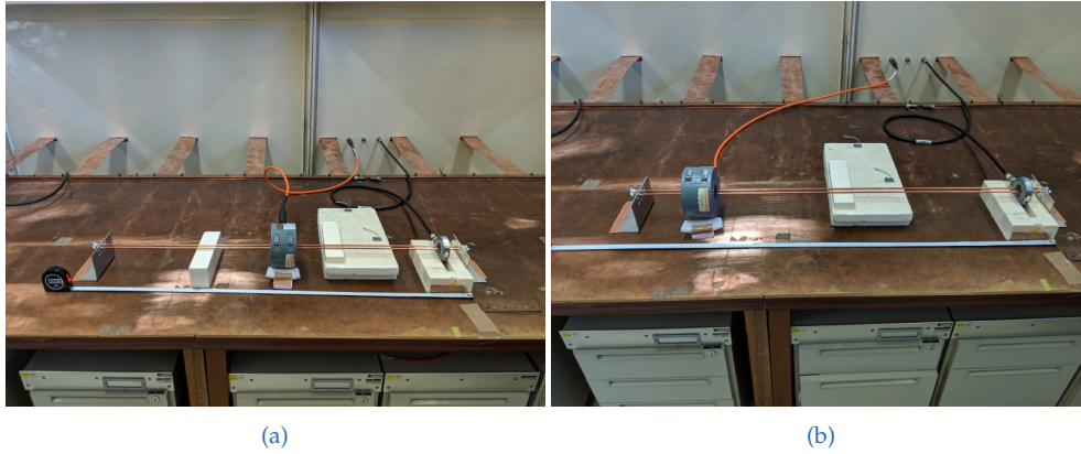
Figure 5.7.: First test setup with the injection and measurement probe at the center (500 mm) and 50 mm from the right (a). Second setup with the measurement probe again at the same position and the injection probe at 850 mm from the right side (b).
