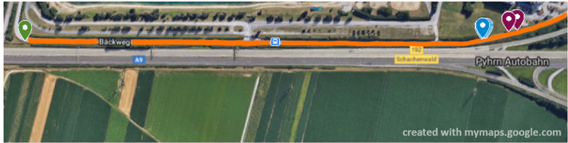
Figure 5.13: Map with the RSU position (green), the cut off points (blue) and the maximum distance points (red)
