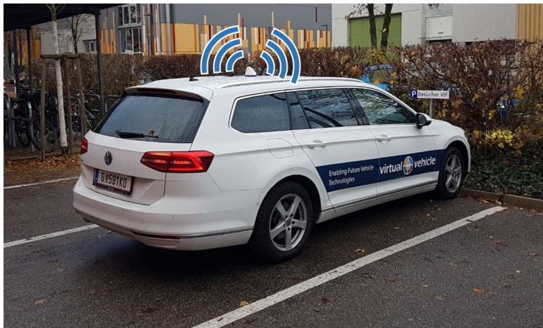
Figure 4.4: Car with Mounted Cohda Antenna on the Roof
