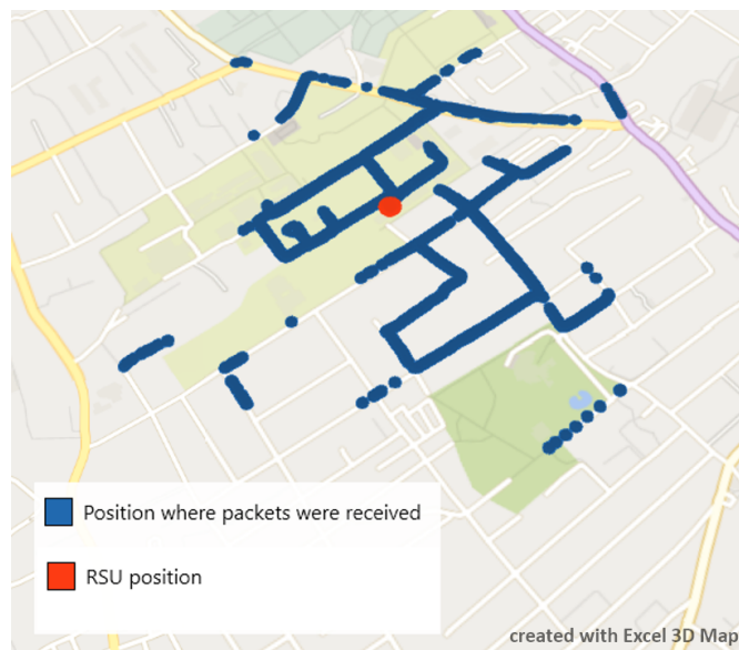
Figure 5.18: Positions where a DENM packet was received with the RSU positioned at the roof
