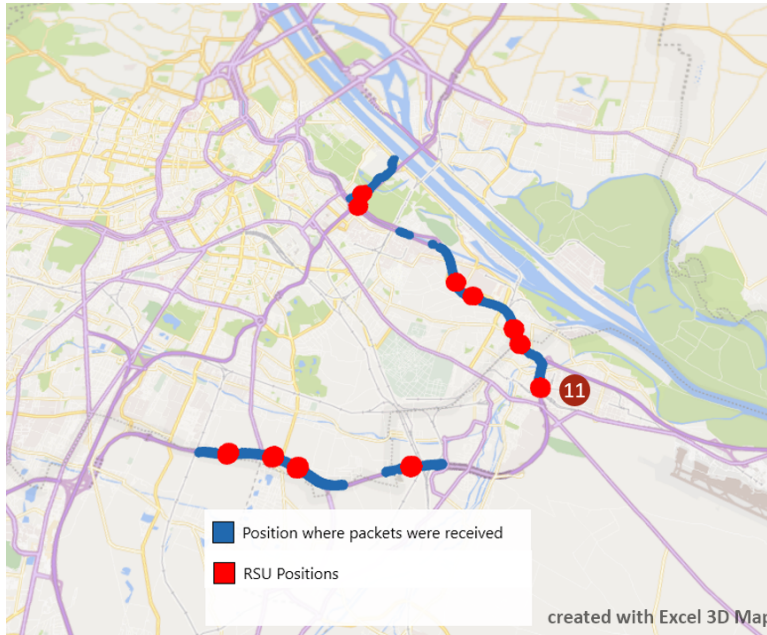
Figure 5.10: The achieved network coverage along the test track on the S1, A4 and A23 around Vienna
