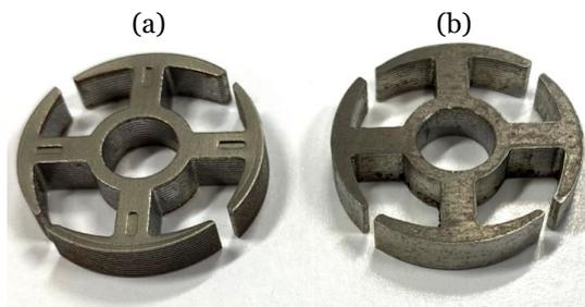
**Figure 3.4:** Photos of the example case drive’s stator package with (a) laminations with mechanical interlockings, and (b) a lamination stack glued with Backlack<sup>®</sup> technology, as illustrated per [56].
