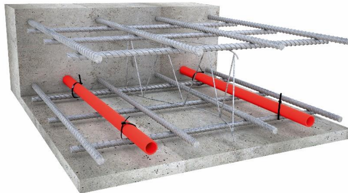
Figure 5. Functional schematic design of thermal component activation: the water-carrying pipes in concrete slabs, walls or floors turn concrete into an energy storage.
