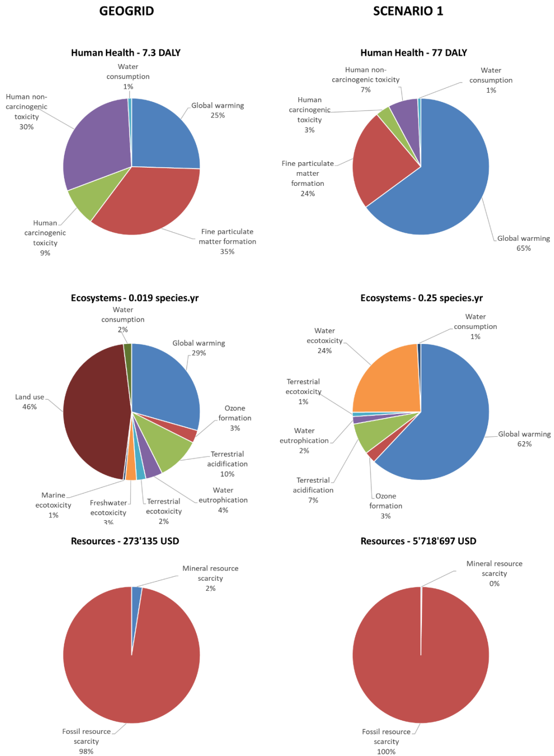
Figure 7a. ReCiPe 2016 v1.04 Endpoint impacts for the energies generated in 20 years by the GEOGRID system and the same amounts from SCENARIO 1.
