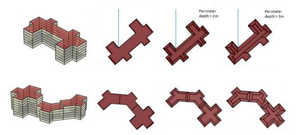
Figure 1. Thermal zoning, single zone and core perimeter zone with 2m and 3m of perimeter's depth. Example for LOD1.2 case (top) and LOD1.3 case (bottom)
