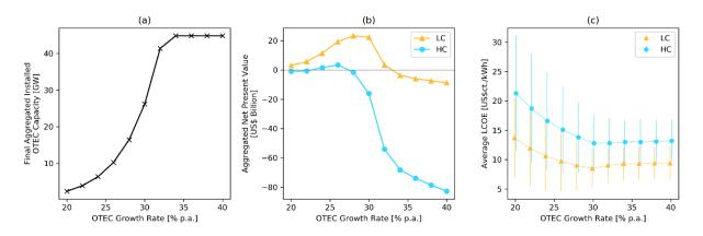
Figure 2 The influence of the OTEC growth rate on (a) aggregated installed capacity, (b) aggregated net present value after 60 years, and (c) average LCOE (error bars show standard deviation). Adapted from (Langer et al., 2021b).
