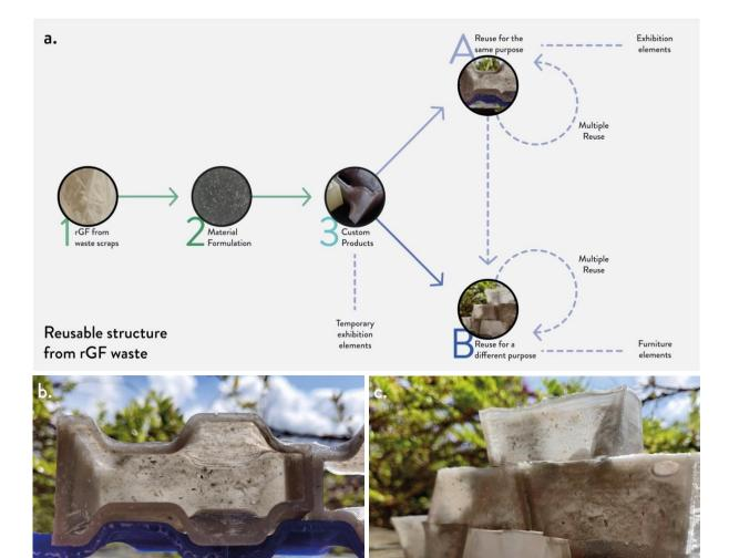
Figure 4. Concept of the reusable custom exhibition – furniture structure from rGFs: (a) concept of the life cycle; (b) detail of the "Brick" single element (1:10 prototype); and (c) possible configuration of the exhibition elements (1:10 prototype).
