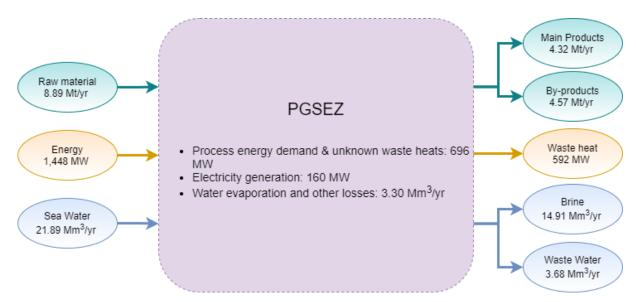
Figure 3 Cluster block diagram incorporating material, energy, and water flows
