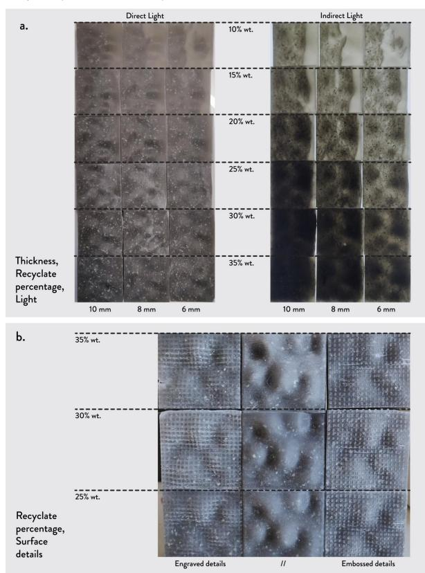
Figure 3. Samples for the preliminary experiential characterization: expressivesensorial qualities related to (a) the thickness, the recyclate percentage and the light variation; and (b) to the recyclate percentage and different surface details.
