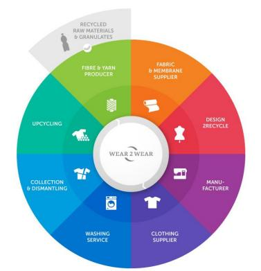
Figure 2. The wear2wear production loop. Starting from the light green field, the fibres are spun either from virgin PES or recycled granulate. The fabric is a three layered laminate just made of PES to guarantee optimal recycling at the EoL, where new fibres are made again from remolten granulate (wear2wear<sup>TM</sup>, 2020).
