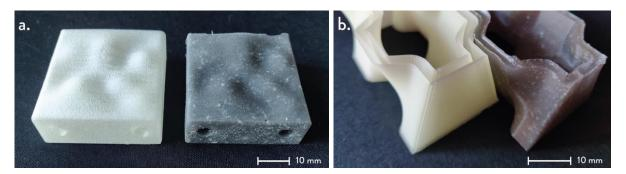
Figure 1. Samples of the 3D printed solvable mould and final shape of the (a) 3D Tiles for the preliminary experiential characterization and of the (b) Bricks.
