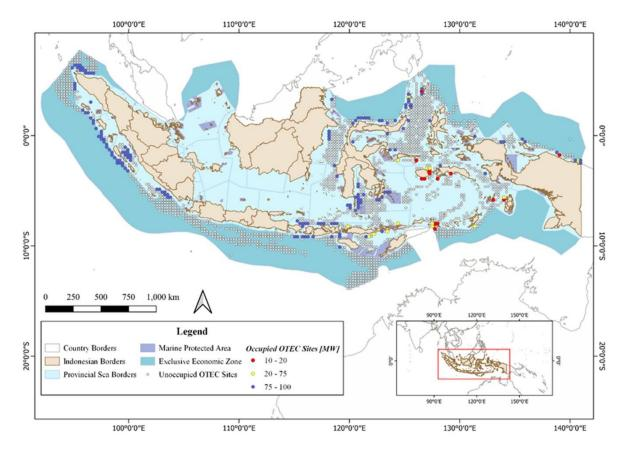
Figure 4 Map of practically suitable and occupied OTEC sites including system size for the economically optimal scenario. Adapted from (Langer et al., 2021b).
