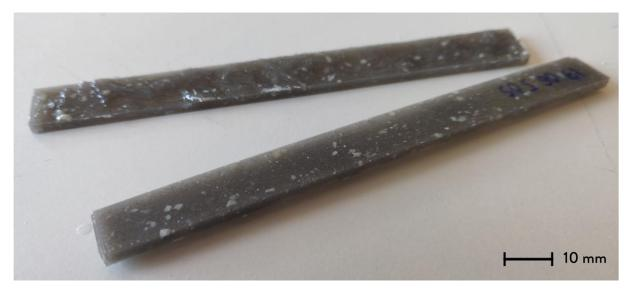
Figure 2. Tensile test specimens with 35% wt. of GF recyclate after the removal of the 3D printed mould according to the ASTM ISO 3039 standard.
