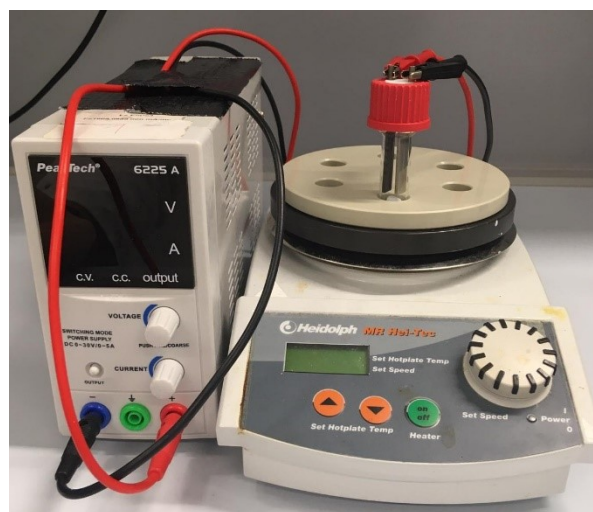
Figure 3: IKA ElectraSyn 2.0 3 and DIY setup
