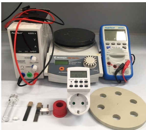
Figure 2: Typical electroorganic synthesis labware and equipment
