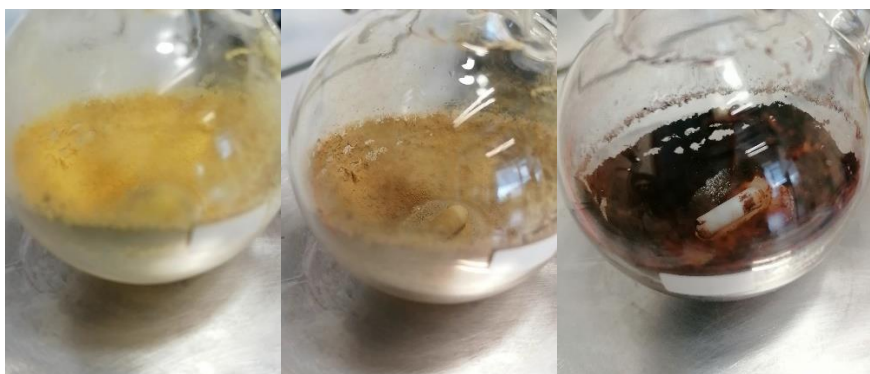
Figure 16: Solid phase reaction of BOC and [L_2MoO_2] at 0, 20 and 120 minutes after the liquid N_2 evaporated.
