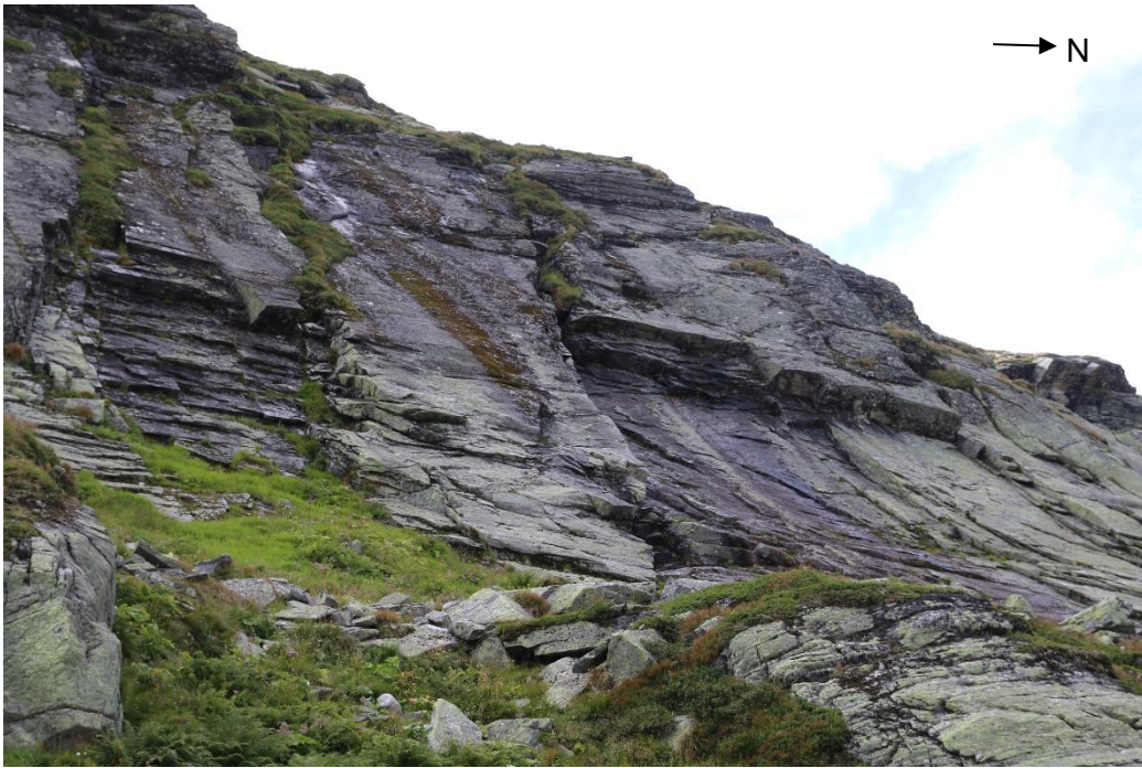
Figure 63 Planar sliding surface on JS1.
