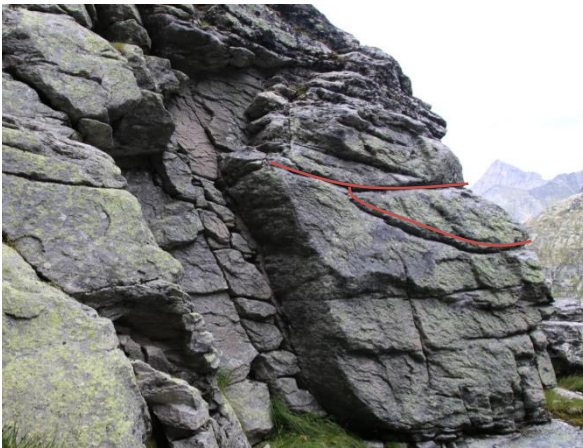
Figure 59 Splay shaped pattern of JS1.
