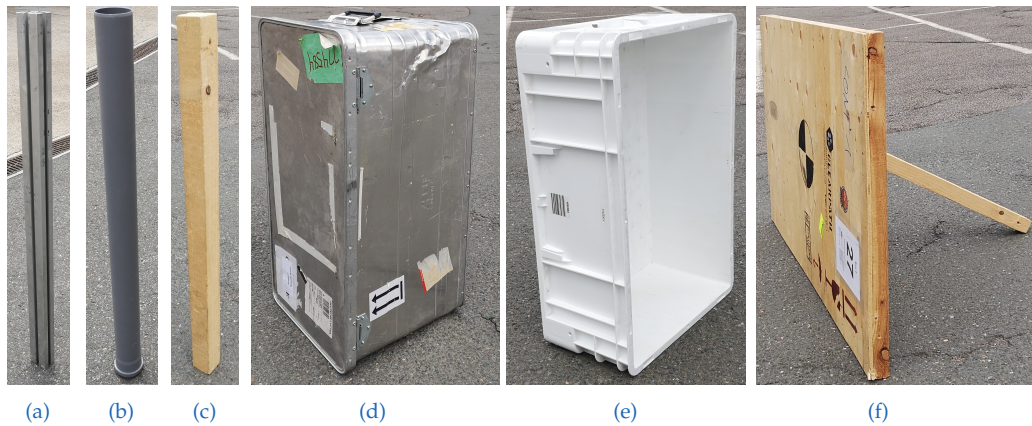
Figure 5.3.: Objects used for the measurements described in Table 5.2. (a) Metal pole; (b) Plastic pole; (c) Wood pole; (d) Metal box; (e) Plastic box; (f) Wood box.
