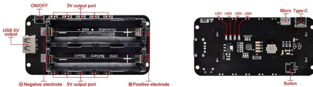
Figure 32: 18650 module in detail [34]
