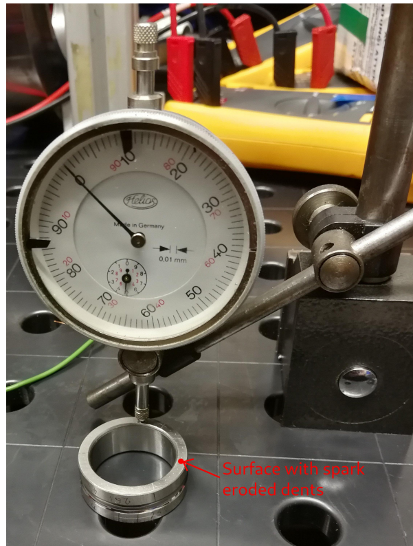
Figure 3.5: Checking if the spark erosion lead to any buildup: No significant signs of buildup were detected.
