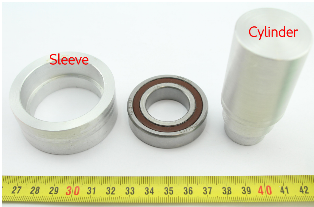
Figure 3.2: Aluminum sleeve and press-out-cylinder for disassembling the bearing.
