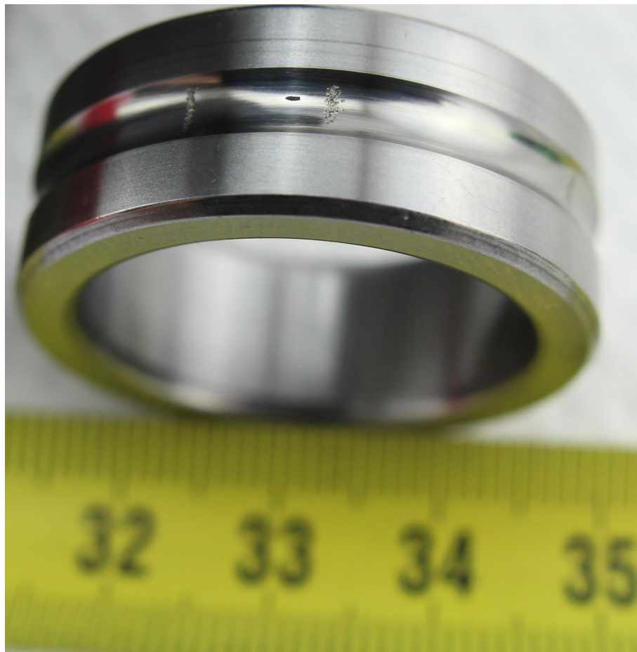
Figure 3.8: Inner ring damage. Three spark eroded spots with parameters: Capacity = 47 \mu\text{F} @32 V.
