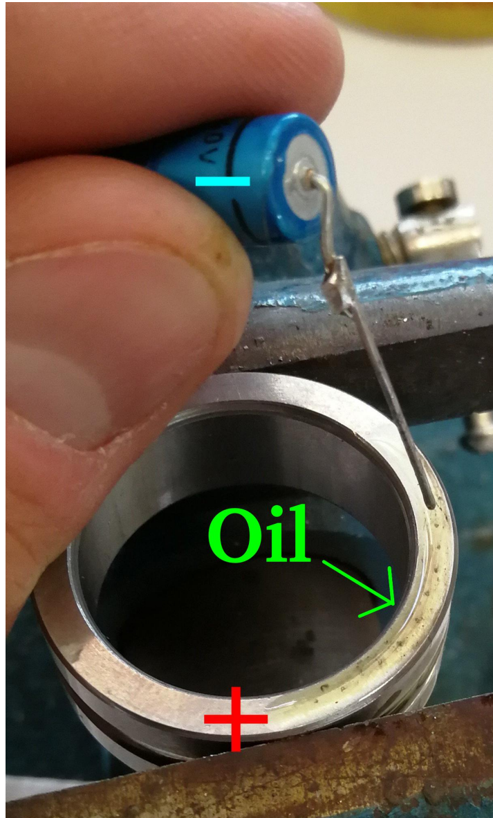
Figure 3.4: Spark eroding test to identify the ideal voltage and capacity values.
