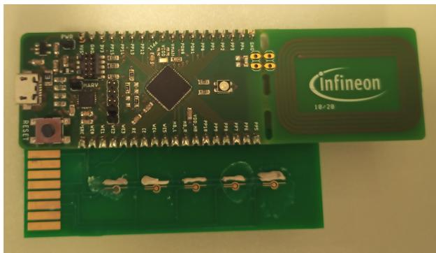
Figure 2.10: Electrodes on PCB connected to the test-chip board
