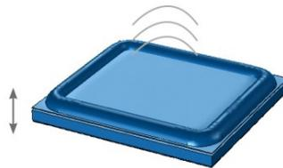
Figure 2.18: Membrane attached to MEMS motor to generate sound, taken from [6]
