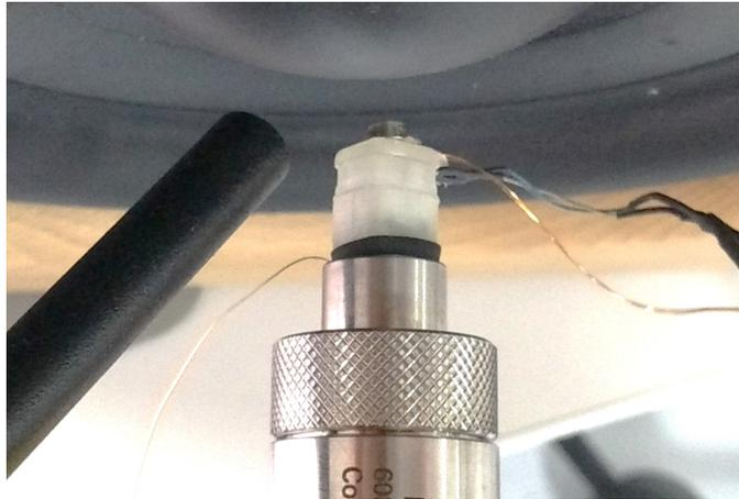
Figure 4.36: Leakage is simulated by placing wire between coupler and eartip
