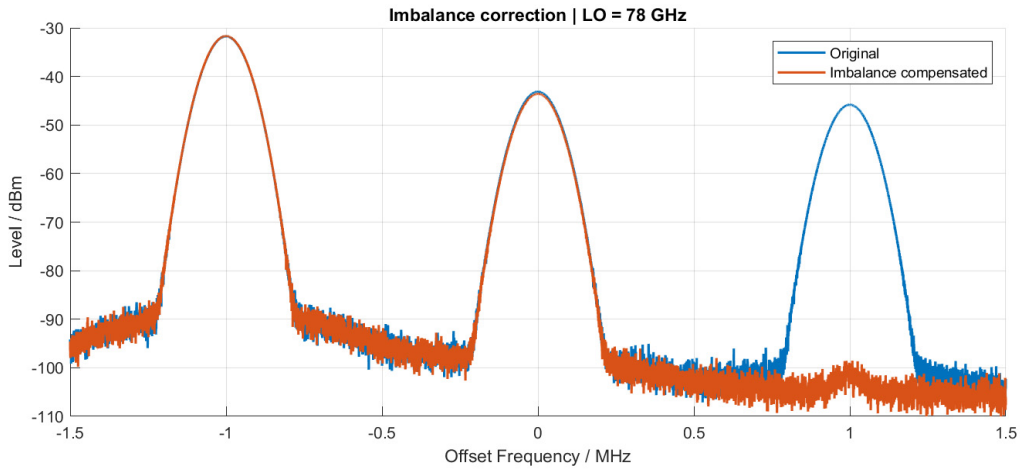
Figure 29: Sideband spectrum after imbalance compensation
