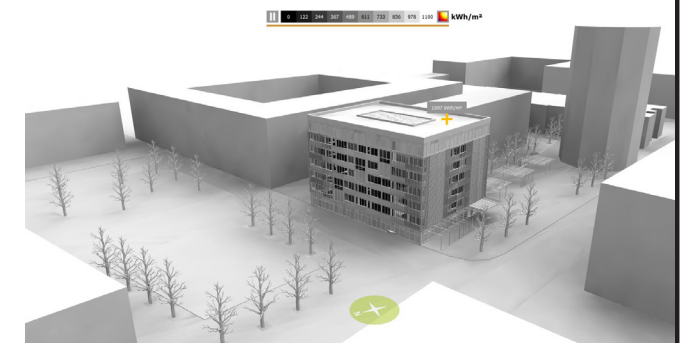
Figure 95. Direct reception ratio of north-west part of the building
