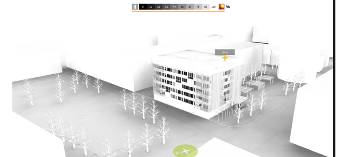
Figure 93. Shading percentage of the north-west part of the building
