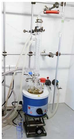
Figure 10: The experimental set-up used for the synthesis of the lithium alkoxide
