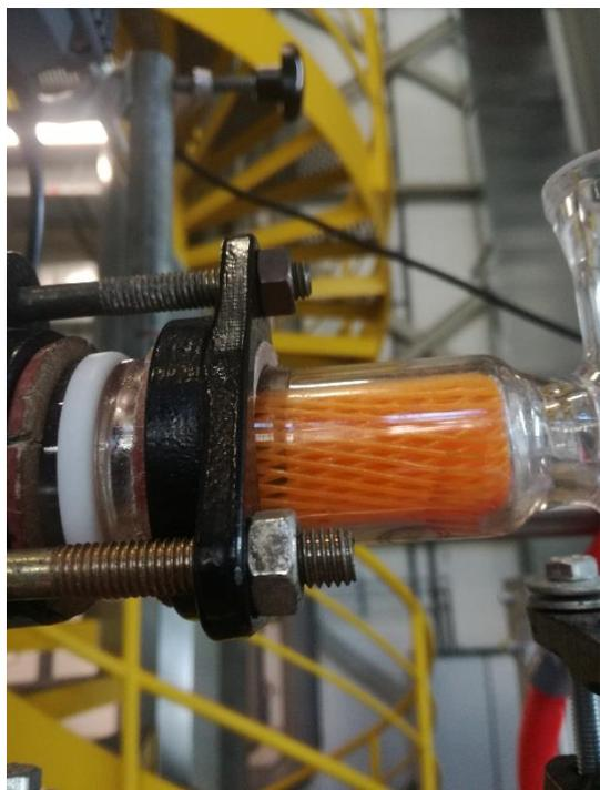
Fig. 3-7: Gas-liquid separator inside the organic phase outlet
