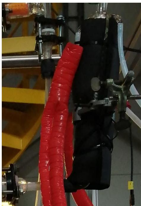
Fig. 3-6: Feed preheater, insulated with ArmaFlex® in black.
