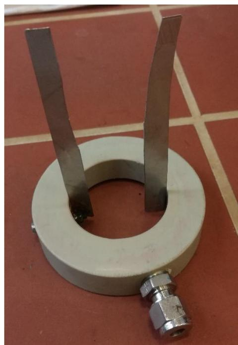
Fig. 3-5: Flow breaker in upside down position, with septum inlet. Baffles made from stainless steel.
