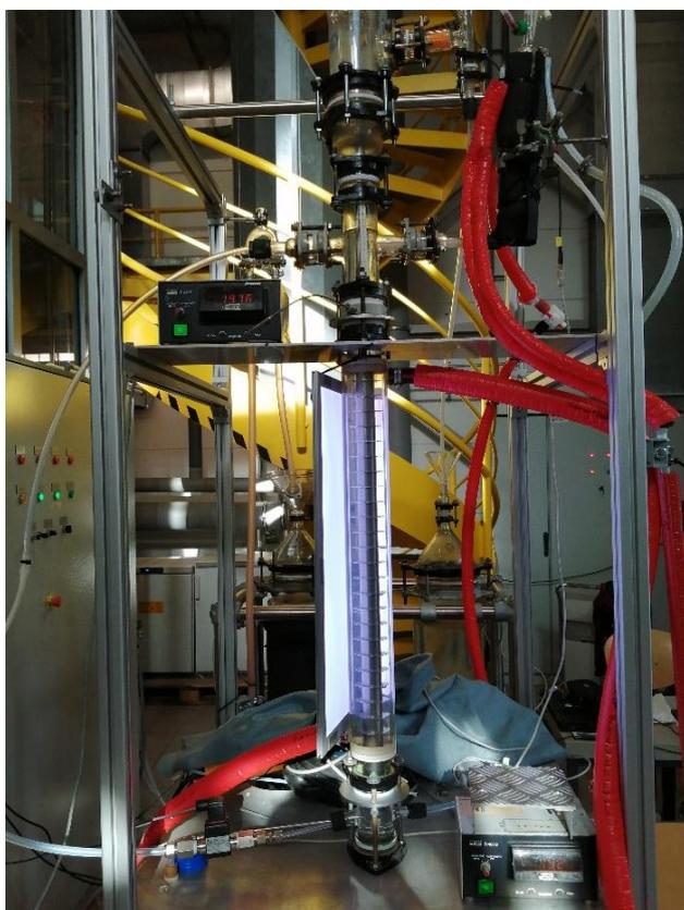
Fig. 3-2: Modified plant used for reactive extraction experiments.
