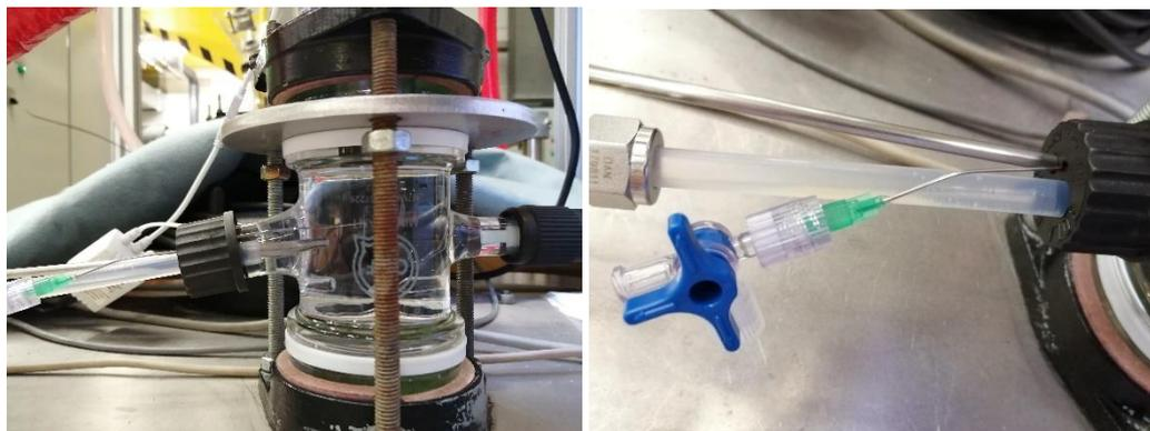
Fig. 3-8: Left: T-piece, Right: Close up view of the inlet for pressure and temperature sensor as well as sample port
