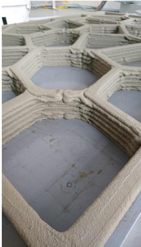
Abb. 15: plug&green, 3D-Printed Prototyp, Ofroom 2017
