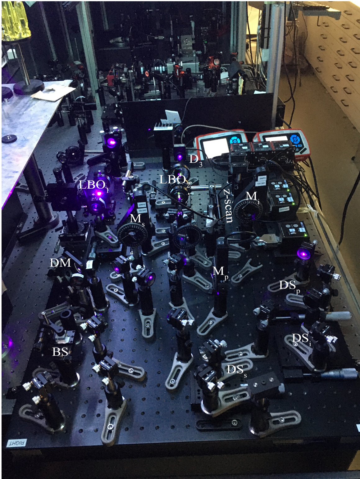
Figure 8.3: The main part of the setup. Red light is sent onto the crystal LBO_1 . A part of the beam is converted into blue light. By a dichroic mirror, the blue light is then spatially separated from the red light. The red beam is then splitted by a 50:50-beam splitter into two beams. Via three translation stages, a spatial and temporal overlap of the three beams inside the LBO_2 -crystal can be obtained. The three motors M_s , M_i and M_p can open or block the specific parts. The crystal is moved back and forth by a motorized translation stage that conducts the z-scans. A thermal powermeter D_3 measures the intensities. The whole movement of the motors and the measurements are controlled by a computer program.
