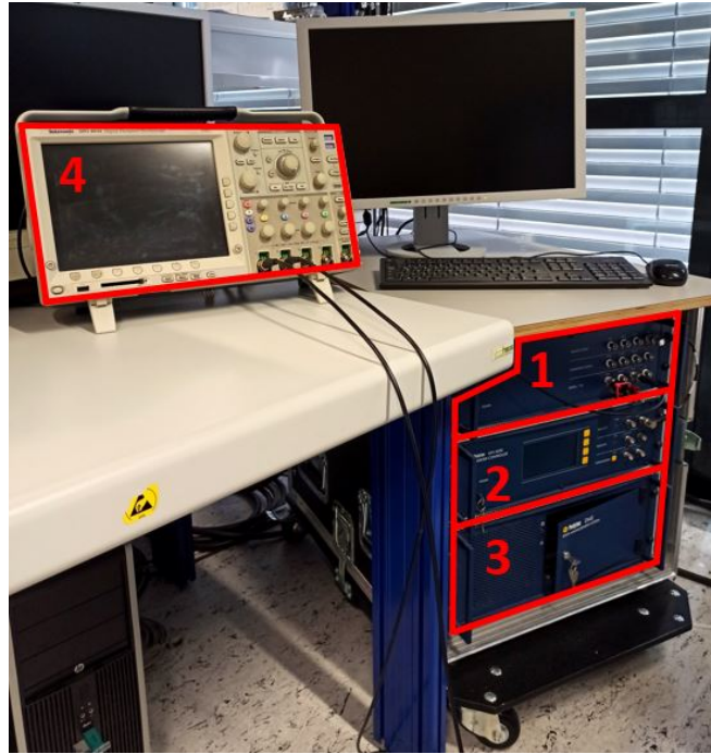
Figure 17: The different components of the LSDV setup. The junction box (1), vibrometer controller (2) and data management system (3) together with the external oscilloscope (4). Although the scanning head is not on the picture, it is the fourth important part of the LSDV setup.
