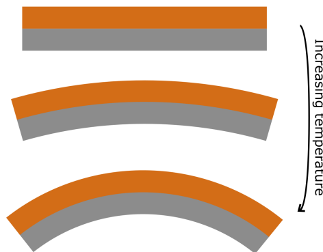
Figure 1: Schematics showing the thermally induced bow of a bilayer system. (substrate (grey) = lower CTE, metallization (orange) = higher CTE)
