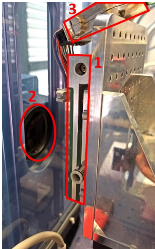
Figure 16: A photograph showing the inside of the HV box. The probecard (1) is mounted on a holder and placed in front of the front lens (2) of the scanning head of the vibrometer. On top of the picture the cable (3), via which the probecard (and its inserted polyheater) is connected with the polyheater setup, can be seen.
