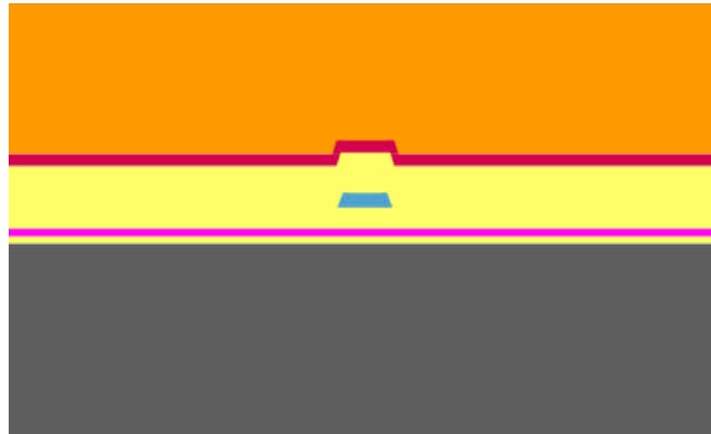
Figure 11: Schematic cross-section of a polyheater (not to scale).
