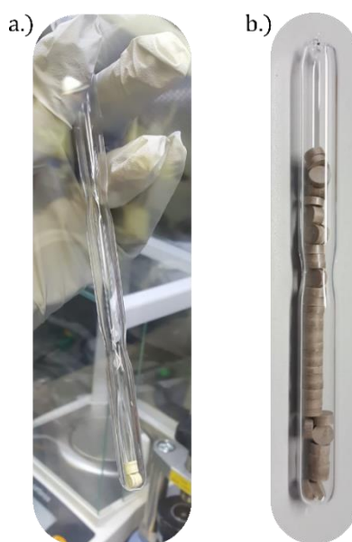
Figure 28: Quartz tubes filled with pressed sample pellets a.) before sealing and b.) after sealing and annealing at 550 °C for 8 h.
