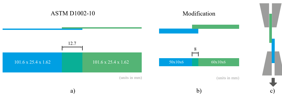
Figure 18: Single lap shear standard dimensions a) ASTM D1002-10 [86] b) standard modification c) experimental setup
