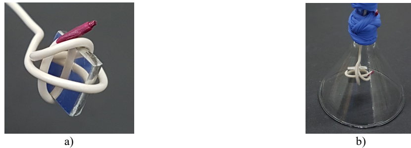
Figure 26: Mg L2+ sample (as-cast) a) ground and wire-wrapped sample b) glass funnel with sealing and placed sample
