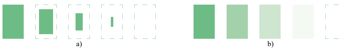
Figure 8: Modes of biodegradation a) surface erosion b) bulk degradation [73]
