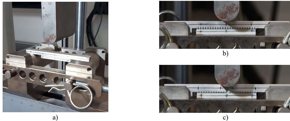
Figure 23: 3-Point bending testing setup a) bending tool b) type 1 c) type 2
